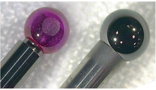
Optical comparison of the tested styli (left ruby, right UltraScanning) Clearly visible: The UltraScanning ball has absolutely no wear.
